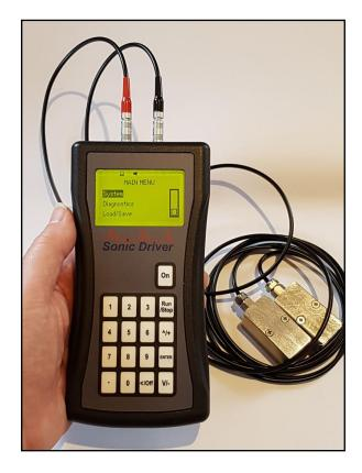
The POCKET-UFM is a light weight, truly pocket-sized instrument. Its intuitive menu driven user interface makes it incredibly easy to use. Its size and the layout of its display and keypad means that it can be operated single handed. Yet all of this is achieved with no compromise in measurement performance. It also incorporates wall thickness and heat quantity measurement functionality.
